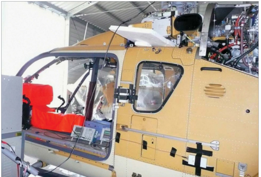
This physical test rig was used to conduct lightning-strike tests of a helicopter at Eurocopter's Donauwörth facility in Munich, Germany. The tests verified the accuracy of Opera FEA models.
