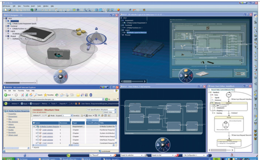
Figure 2: The mapping of allocations between parameters on physical parts to requirements on functional and logical models in Teamcenter, enables the use of independent groups of parts in the design of multiple products.
