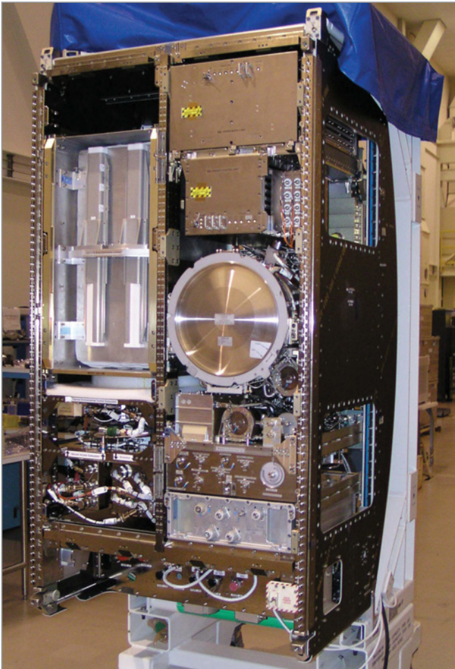
MSRR-1 in launch configuration. The right side of the rack contains the MSL Engineering Model. The left side contains the MSRR-1 Rack Support Subsystems (lower portion) and the stowage container (upper portion). The left side has the accommodations/interfaces to support an additional furnace module if required.
